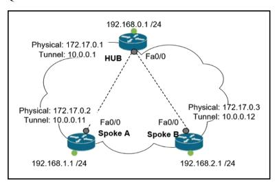
Refer to the exhibit. Which interface configuration must be configured on the HUB router to enable MVPN with mGRE mode?
