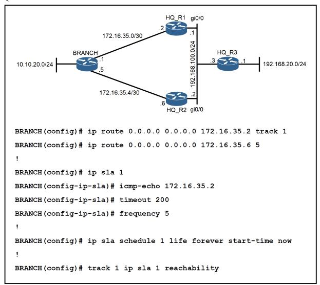
Refer to the exhibit. An engineer has successfully set up a floating static route from the BRANCH router to the HQ network using HQ\_R1 as the primary default gateway. When the g0/0 goes down on HQ\_R1, the branch network cannot reach the HQ network 192.168.20.0/24. Which set of configuration resolves the issue?
